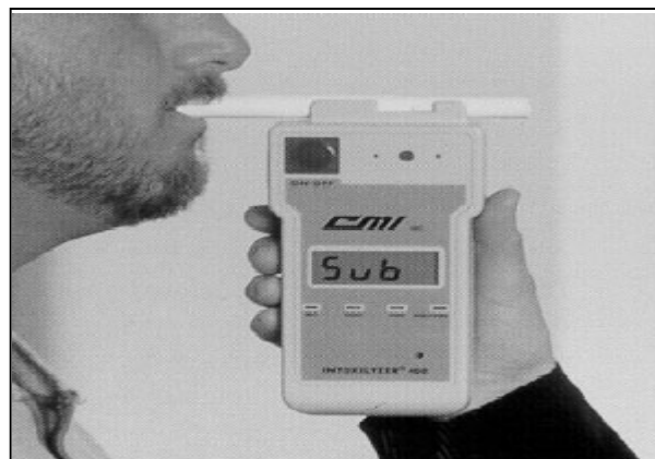
The IntoxilyzerPA 400D, used by the Edmonton Police Department, is a screening device with a built in processor which stores data of tests and refusals — a feature which police do not utilize.
